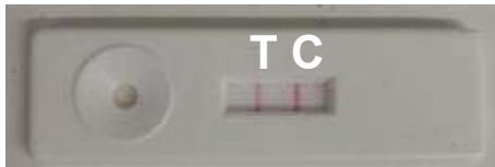
Figure 10. Positive result indicated by red line under 'T' (first) and the control line 'C' (second), in a Phytophthora lateral flow device (LFD).
